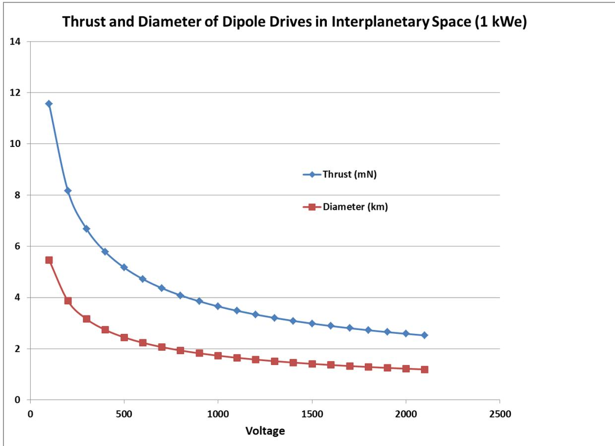
*Fig. 3. Thrust and Diameter of a 1 kWe dipole drive system operating as a thruster in interplanetary space. For comparison, a 2 kilovolt dipole drive acting as a solar wind sail with a diameter of 1 km would use no power and generate drag/lift force of about 2 mN at 1 AU.*
