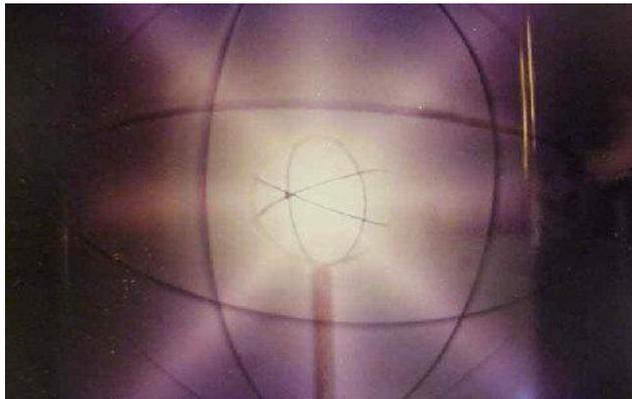
Fig. 7 Photograph of a fusor in operation.
