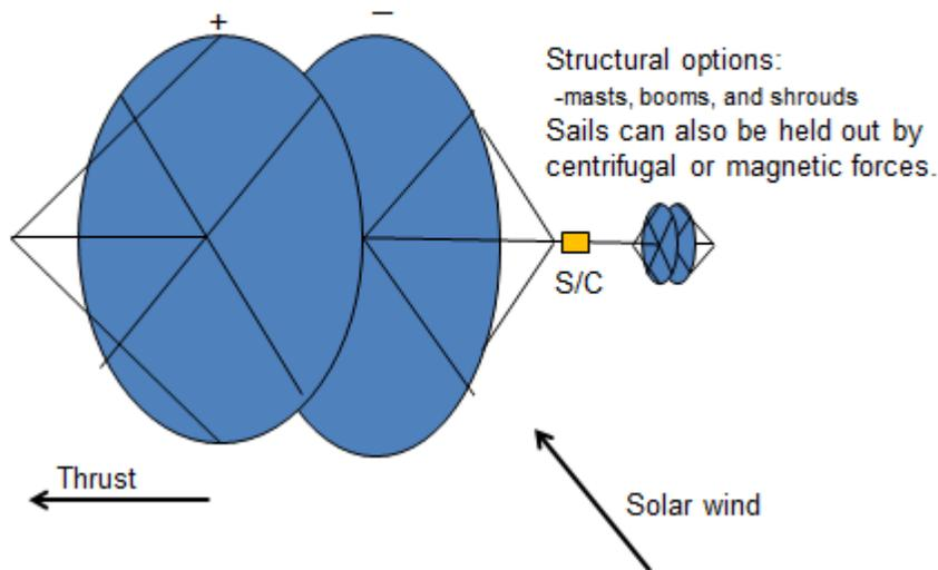
*Fig. 6. Options for dipole drive spacecraft configuration. Small dipole drive systems can be used for attitude control.*
