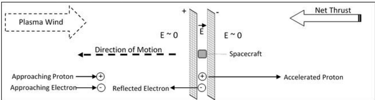
**Fig. 1. The Dipole Drive Accelerating within a Magnetosphere. Power is required to fire electrons to match the accelerated proton jet.**
