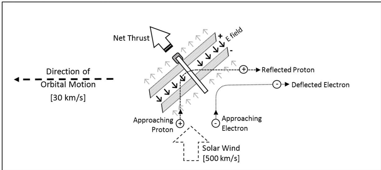
**Fig. 2 The Dipole Drive Operating as a Sail in Interplanetary Space. The protons are reflected by the strong positive field between the screens, while the electrons are reflected before they can reach this region by the weak electrical field outside the screens. The drive thus acts as a sail reflecting a one-fluid plasma. No power is required.**
