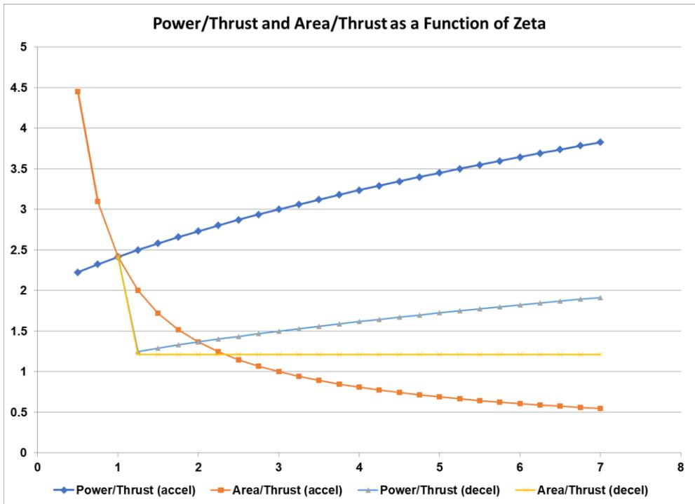
Fig 5. Relative Power/Thrust and Area/Thrust as a function of  $Z=(\text{engine voltage})/(\text{kinetic voltage})$ . There is a step factor of 2 increase in thrust during deceleration when  $Z$  reaches 1, because protons are reflected. For acceleration,  $\text{Power/Thrust} \sim 1 + \sqrt{1+Z}$ , while  $\text{Area/Thrust} \sim 1/(-1 + \sqrt{1+Z})$ .
