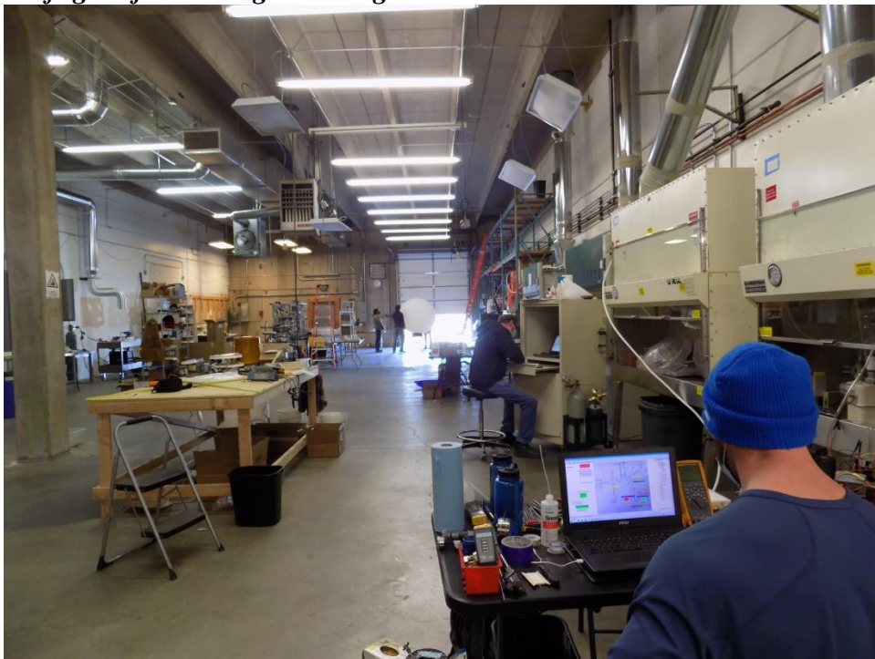
The balloon was inflated through a long tube 30 meters away from the GRS, as it would be done in flight. In mid-ground, GRS PI Mark Berggren takes a gas chromatograph sample to verify dissociation. Measurements showed consistent 99.8% conversion of ammonia to nitrogen/hydrogen mix throughout the inflation process.
